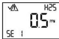
One sensor Installed
