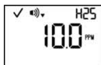
Low alarm setpoint
