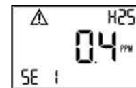
Single sensor data failure
