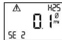
Single sensor zero failure
