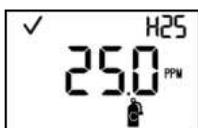
Calibration gas setpoint
