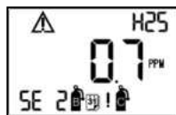
Single sensor bump failure with calibration overdue
