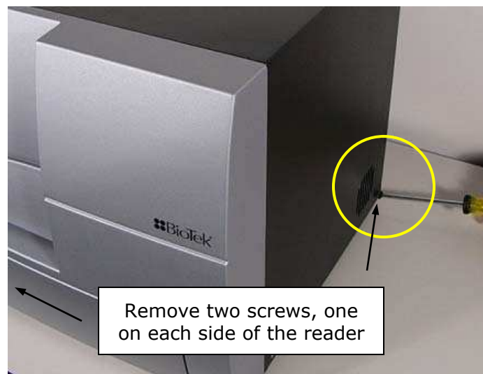
Figure 2: Removing the two side screws.
