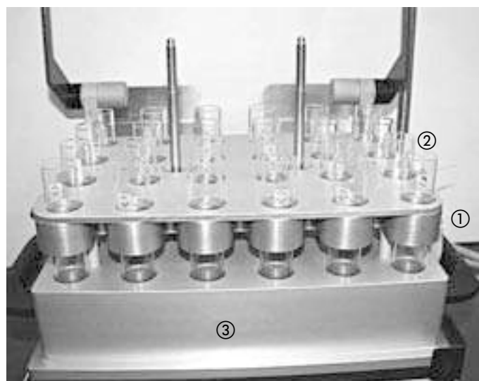
Figure 40: Reflux modules on rack R-24 with test tubes
