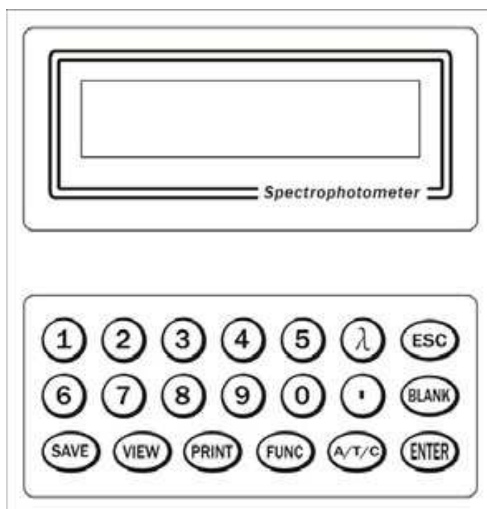
Figure 2: Keyboard and display layout
