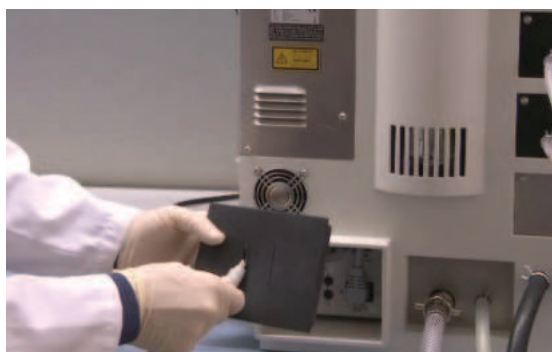
Fig. 5.10: Guidance of the cable through the cut-out
