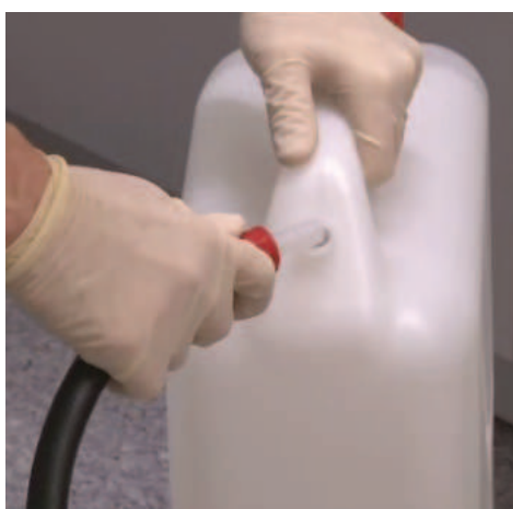
Fig. 5.7: Connection of the drain hose using the straight connector
