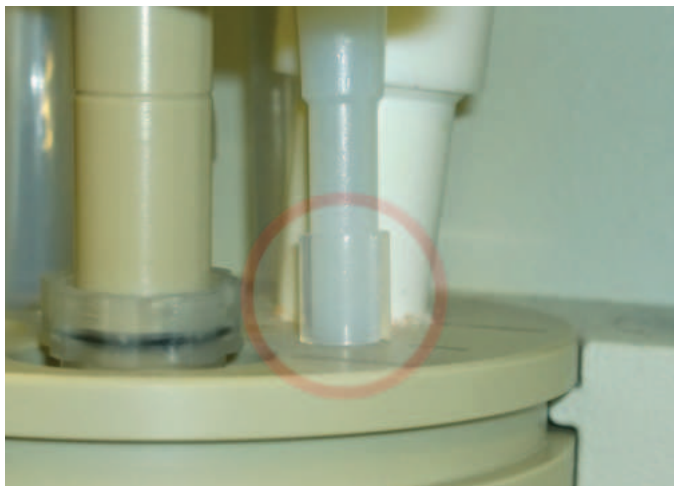
Fig. 5.12: Mounting of the spacer at the dosing tip
