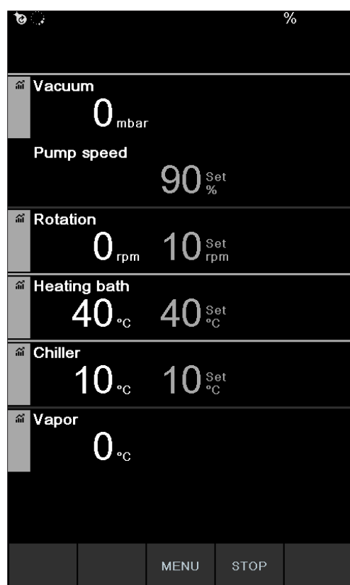
Fig. 42: Continuous pumping for drying the system started
