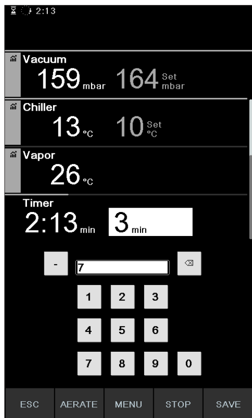
Fig. 37: Editing parameters while distillation is in progress
