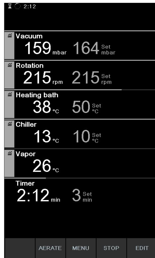
Fig. 36: "Timer" screen while distillation is in progress
