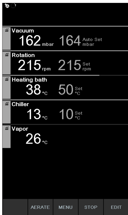
Fig. 45: Information displayed during automatic distillation
