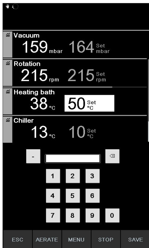
Fig. 33: Editing parameters while distillation is in progress
