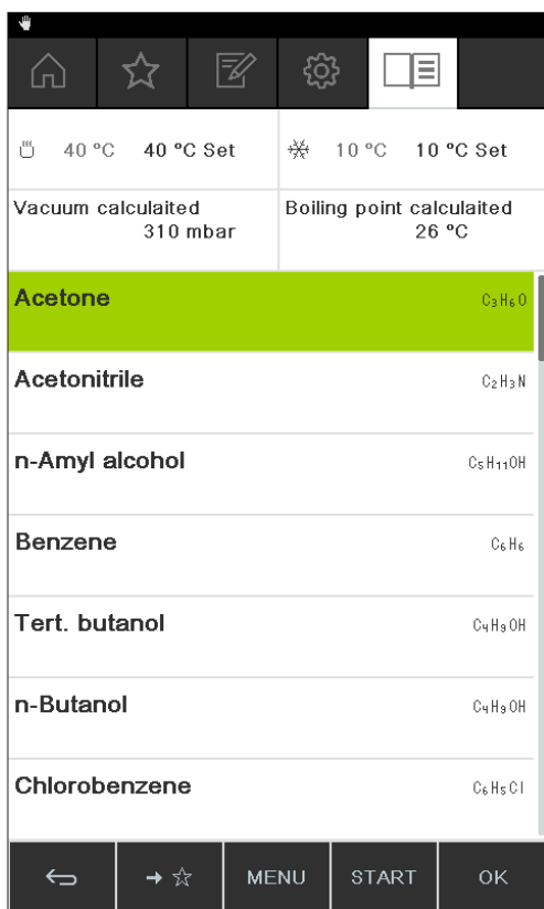
Fig. 60: Selecting "Set" temperature for heating bath when using equipment of a different make
