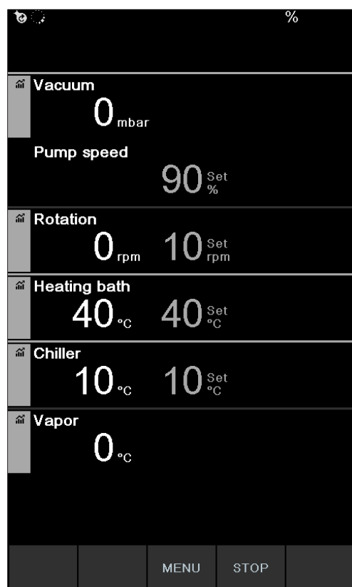
Fig. 43: Continuous pumping for drying the system started
