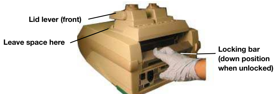
Figure 4. Inserting the reaction module into the bay.
