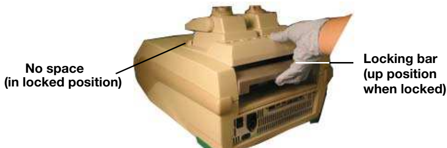
Figure 5. Locking the reaction module in place.
