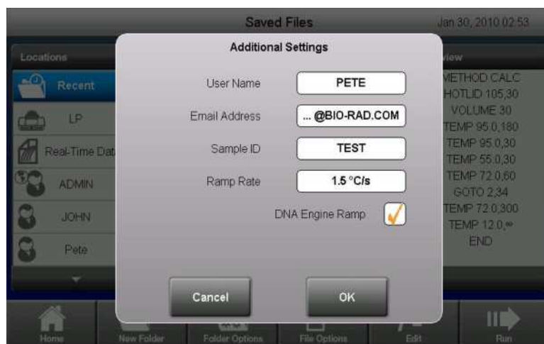
Figure 20. Add additional settings to your protocol including running in DNA Engine Ramp mode and sending an email notification upon run completion.
