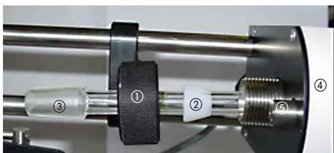
Fig. 19 : Assembly/disassembly of the vapor duct
