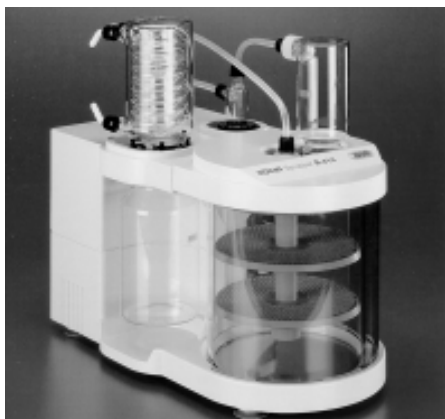
Fig. 8: B-414 scrubber with cold trap and collecting vessel, 1.2 litre
