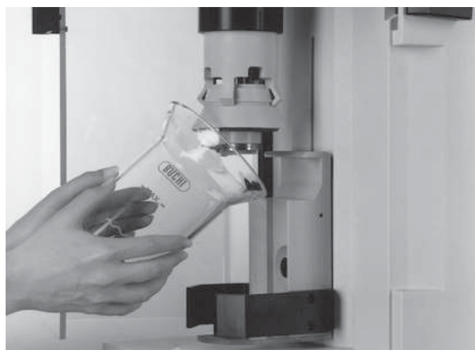
Figure 7: Inserting the sample beaker
