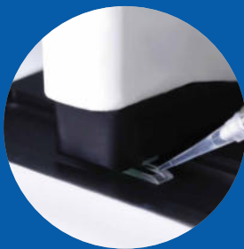
Load Cell Suspension into Sample Chamber
