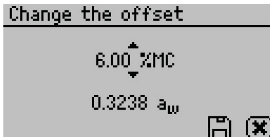
Figure 20 Adjust the moisture content value to match the reference method
